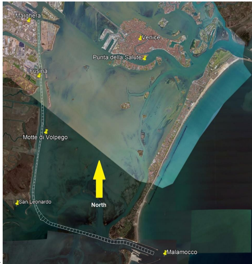
Figure 9 Mesh adopted for the spatial discretisation of the optimized MMC. Image ©Google Earth.
