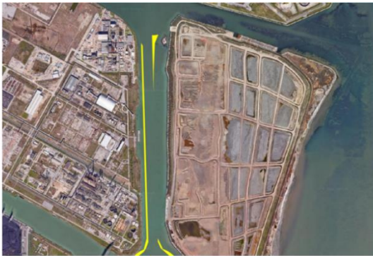
~ 10 m widening of the channel (west side, close to berth) between Turning Basins n°4 and n°3
