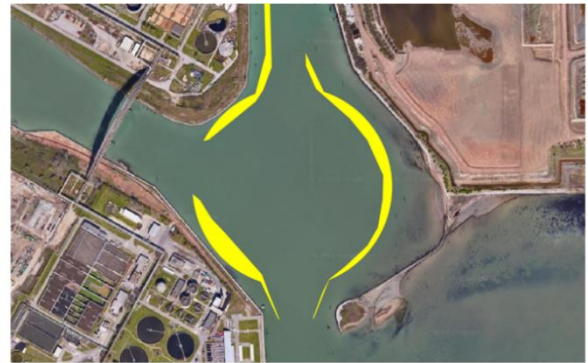
Improvement of Turning Basin n°4 (local widening, generally between 10 and 30 m) to match the original diameter indicated in the Port Regulatory Plan
