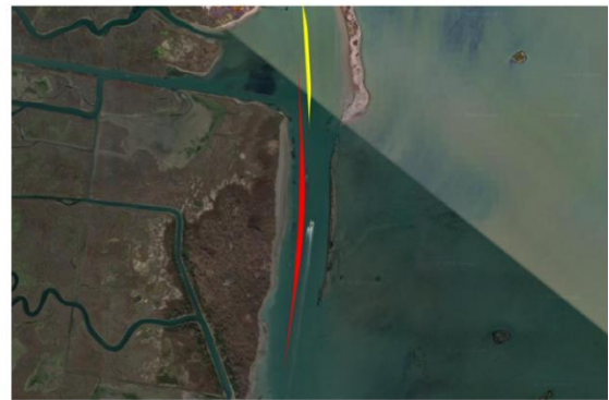
Partial rectification of the Channel (max widening locally in the order of 40 m)
